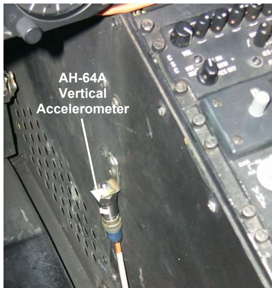
Figure 4. Vertical Accelerometer Installation (External Wiring)
