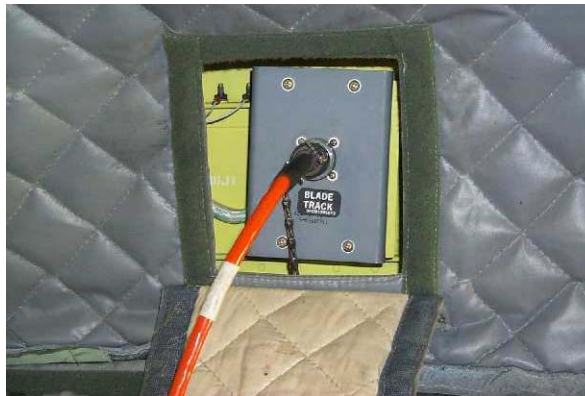
Figure 4. BLADE TRACK Bulkhead Receptacle near STA 256
