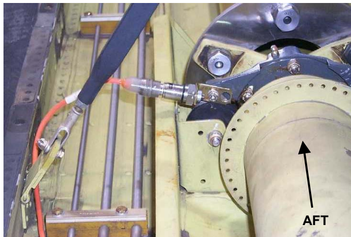
Figure 10. Typical Hanger Bearing Installation
