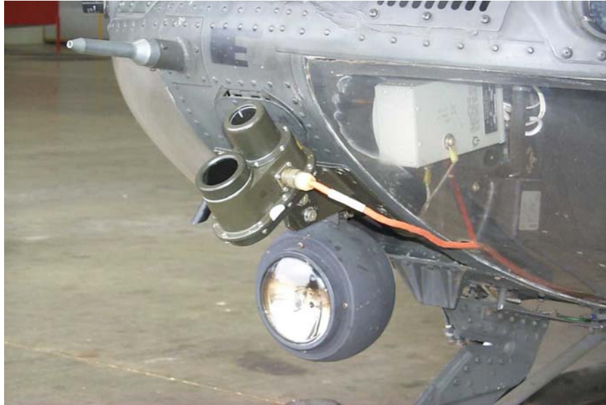
Figure 5. Universal Tracking Device (UTD) Installation
