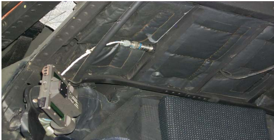
Figure 3. Lateral Accelerometer Installation (SPU/External Wiring)
